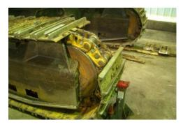
6. Assemble the **Tracbuster 2000**© with the cylinder rod facing towards the press frame and torque the assembly bolts to 200 ft-lbs.
