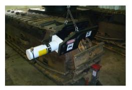
9. Hang the **Tracbuster 2000**© over the master pin at the proper angle, with the cylinder in straight alignment with the link and pin, and anvil centered over the opposite end.
