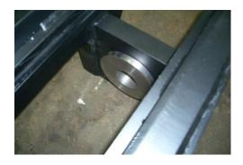
Due to normal wear and tear, anvils may need to be occasionally de-burred to allow for a more consistent inside.
