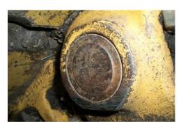
4. Move the machine to position the master pin about 20-30 deg from the vertical center line of the idler. At the same time block track just under the idler high enough to keep the track from falling to the ground when the pin is removed.
