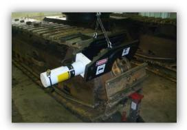
9. Hang the **Tracbuster 1500**© over the master pin at the proper angle, with the cylinder in straight alignment with the link and pin, and anvil centered over the opposite end.
