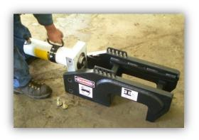
7. Choose the largest anvil possible to bring the chain link as close to the cylinder as possible.
