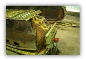
5. Remove two pads, one on each side of the master pin.
